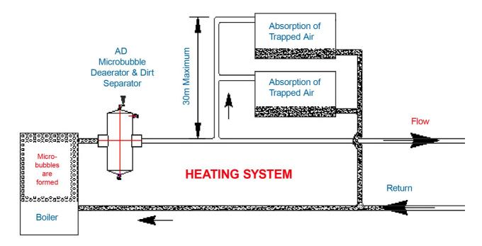
In cooling systems this should be in the return. The AD should always be installed before equipment that needs protection from dirt, sludge, etc., (ie. Chillers, controll valves, pumps, etc.) In existing systems where there are problems with dirt, sludge, etc. a demountable unit should be installed, our AD-R will solve this problem. This applies to in and around the plantroom where new chiller unit and control equipment have been installed but the existing system has been left intact.
